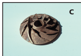
Figures 5A) a worn semi-open impeller; 5 B) the pump shaft to which the impeller(s) is attached can be adjusted by turning the nut at top of the gear head; and 5C) sheared impeller resulting from an improper adjustment. An adjustment should only be done by a trained professional.
