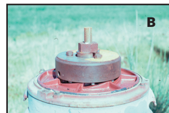
Figures 5A) a worn semi-open impeller; 5 B) the pump shaft to which the impeller(s) is attached can be adjusted by turning the nut at top of the gear head; and 5C) sheared impeller resulting from an improper adjustment. An adjustment should only be done by a trained professional.
